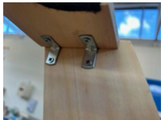
Figure 49: metal brackets joining the frame
