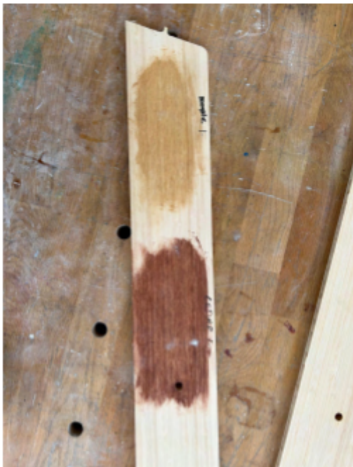
Figure 52: Bamboo wood with maple stain (top) and cedar (bottom)
