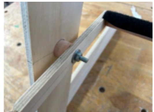
Figure 47: bolts joining rails to the frame
