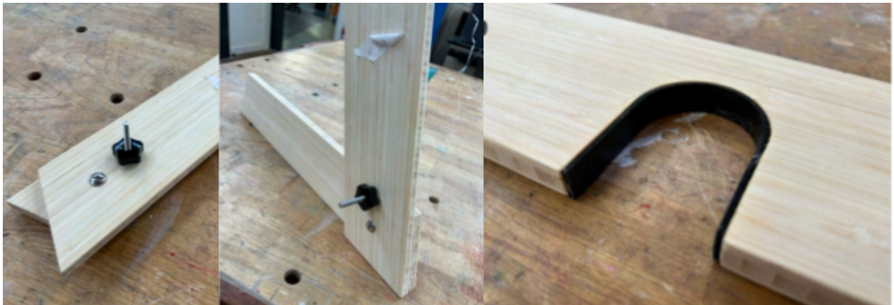
Figure 56: locking pins holding the leg folded down (left) and extended (right)
