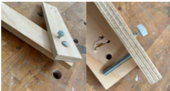
Figure 54: failed spring plunger, the plunger was too small and consequently too weak to stop movement of the two pieces on a demo that was made.
