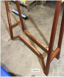
The part of my project I am most proud of is the compound angle legs which required a lot of maths to work out angles as well as the best way to make the angles to make sure they support the project. The angles of the legs add a unique design and an extra complexity feature to make it stand out.
