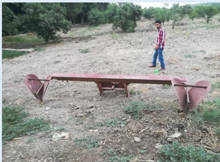
The plough purchased by farmers (on self-help basis) to develop water channels in citrus orchard
