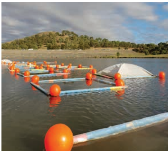
Aquatic mesocosms (experimental enclosures) in place in Lake Tuggeranong, investigating potential control measures for blue green algal blooms. (Photo credit: Ross Thompson)
